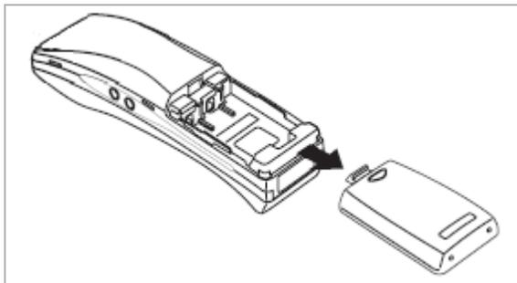
2. Connect the battery pack connector, observing correct polarity to the jack inside the battery compartment, as shown on the right.
